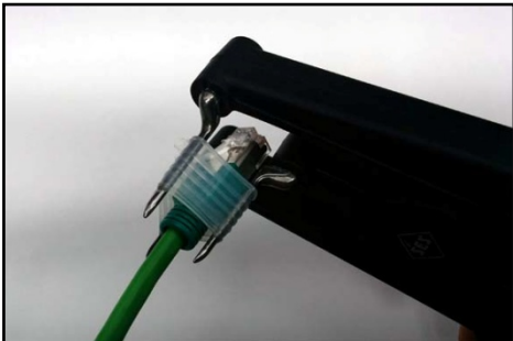
FIGURE 14 - INSERTING RJ-45 END THROUGH SHROUD
