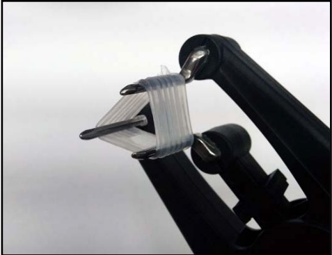
FIGURE 13 - SHROUD STRETCHED WITH TOOL
