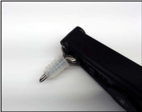
FIGURE 12 - PROTECTIVE SHROUD PLACED ON TOOL
